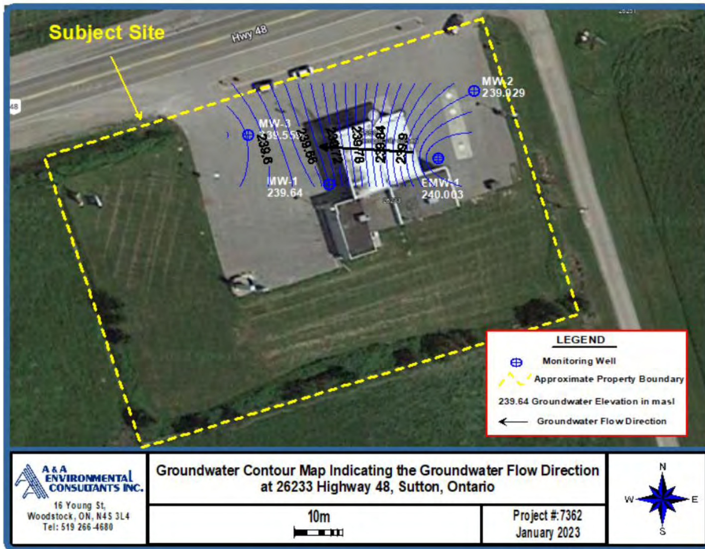
Figure 6 – Groundwater Flow Direction
